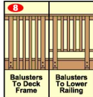
9. Measure the distance between each set of posts. Calculate the number of balusters you will need to maintain an equal distance between all balusters. Remember the balusters should be no more than 6" apart. Mark the location of each baluster on the top railing and lower railing or joist.
