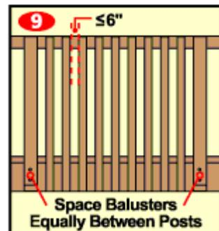
10. Measure and cut the balusters to length. For an attractive appearance, cut the bottoms of the balusters at a 45-degree angle. Using 2 screws at the top and 2 screws at the bottom, install the balusters.
